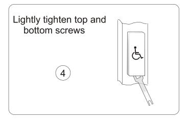
We recommend leaving a tightening tool inside the door header for the next person that needs to remove the switch.
